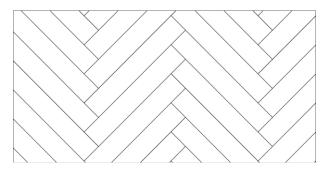
Chevron: There are left and right planks/elements which are alternately located in the package. A stainless cutting rail/steel strip will help you to put on the first row. Care must be taken to ensure that this is exactly in place and direction.
